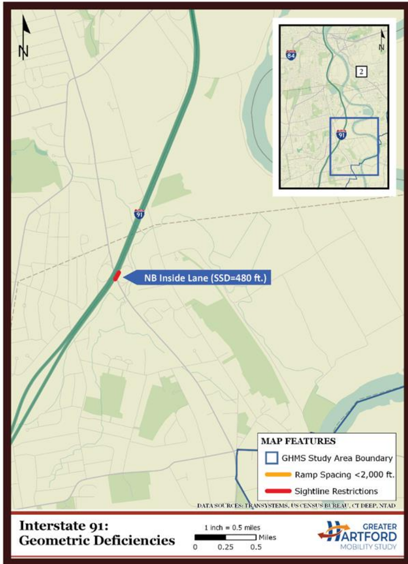
Figure 3-5: Identified I-91 Deficiencies
